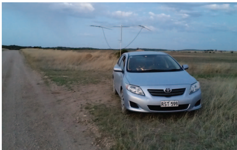
The VK5APN portable EME antenna has worked many stations throughout the world.
