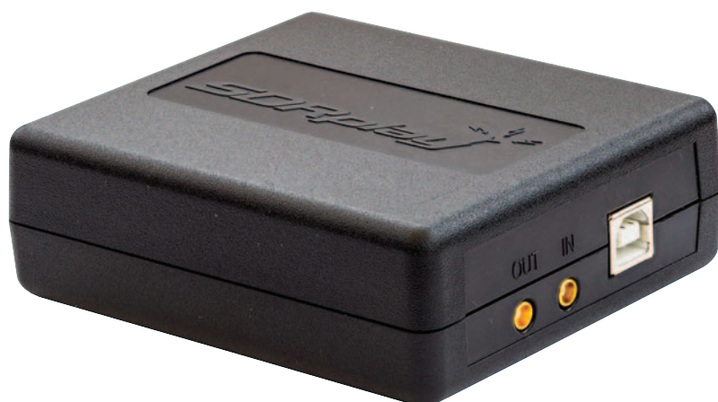
PHOTO 2: Side view of the RSP-2 showing USB connector and MCX coax clock in and clock out ports.
