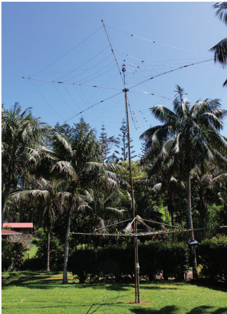
The team used a rotary clothes line and bamboo to support one of their hex beams.
