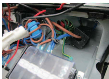
PHOTO 5: RF interference suppression cores in an air source heat pump
