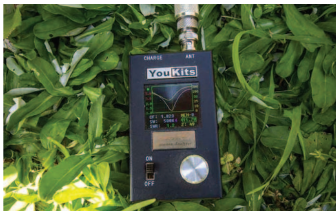
The analyser shows the excellent match with the DJ0IP-inspired top loaded 160m inverted L.
