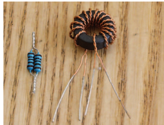
PHOTO 1: Balun made for the return loss bridge, plus two hand-picked 100Ω resistors paralleled to give as close to 50Ω as possible.
